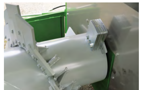
15 mm shaft width with 3 fixed screws. The balanced axle ensures long life.
