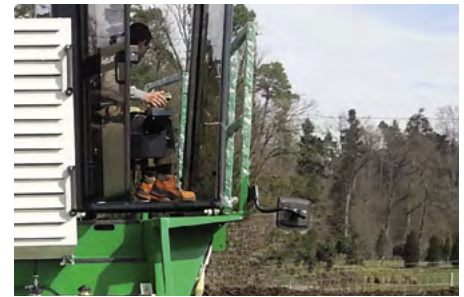
Exterior mirror for optimal view of the roller
