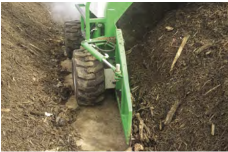
Single swiveling, hydraulic shields ensure clean troughs.
