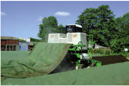
Fleece roller hydraulically height-adjustable with quick-change system
