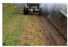
Thanks to the swivel weight it is also possible to move through the field. It also ensures optimum weight distribution and reduces the overall weight by approx. 1'500kg.
