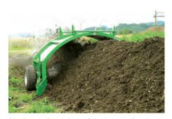
Maximum dimensions of the battery: 3 x 1.5 m, so that it can be composted aerobically.
