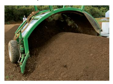
The TG 301 is a compost turner that is easy to use, mechanically operated, stable and maneuverable with optimal weight distribution. It is ideal for field-edge composting, small composting plants and organic farms with compost production up to 6,000 tons per year.
