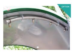
Water sprayer with nozzles. To achieve an optimal microorganism climate within the mound, the addition of water is essential.
