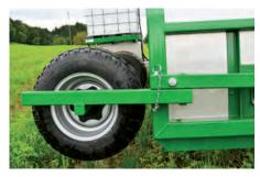
For transportation, the support wheel can be pivoted away, disassembly is not necessary.
