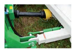
Direct drive - transmission om transfer shaft
