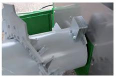
12 mm shaft width with 3 fixed screws. The balanced axle ensures long life.
