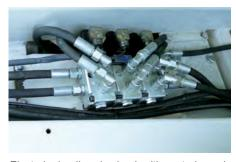
Electrohydraulic valve bank with control panel; (Single, double or triple)
