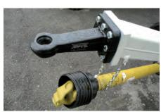
Standard trailer hitch front: DIN coupling
