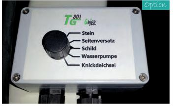
Easily managable control panel. Switching via solenoid valves.
